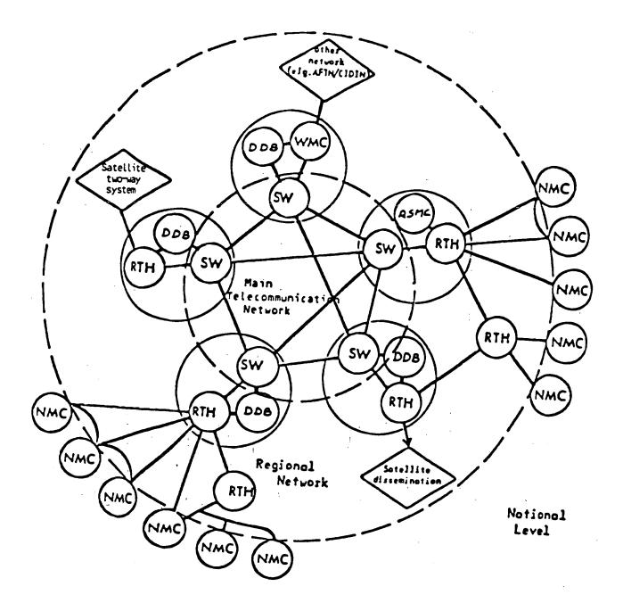
SW: Switching Node (included in functions of RTHs on the MTN)
