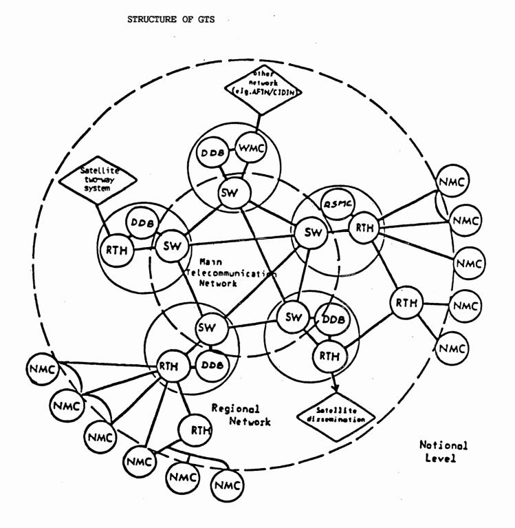
SW: Switching Node (included in functions of RTHs on the MTN)
