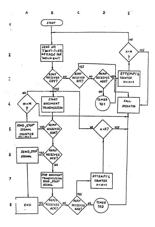
Figure 1 - The algorithm of operation of the transmitting centre
