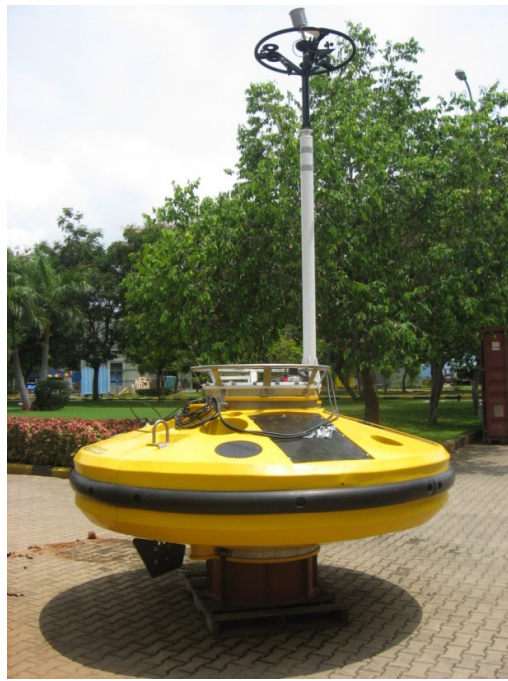
Fig. 6.1 ASSEMBLED BUOY FOR BURN IN TEST
