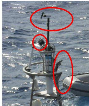
Figure 12. Brazilian PIRATA Buoy (ATLAS) Showing Component Removal
