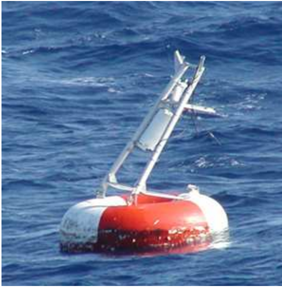
Figure 3. Ship Collision Damage to TAO Buoy
