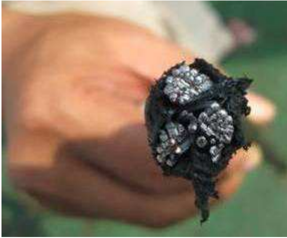
Figure 14. Cut Cable – Indonesian Tsunameter
