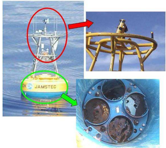
Figure 15. Theft of Met Sensor and Electronics Payload – TRITON Buoy
