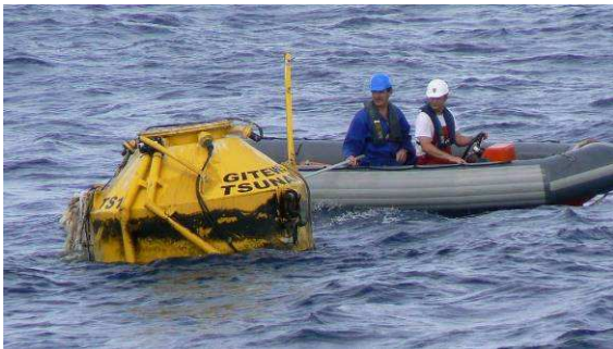
Figure 18. German GITEWS Tsunami Buoy – Stolen Superstructure and Buoy Payload
