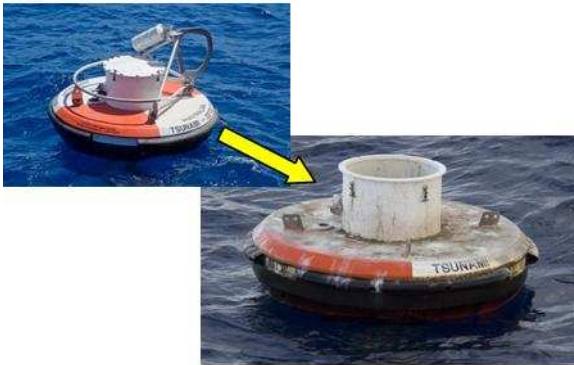
Figure 16. Australian Tsunameter - Stolen Superstructure and Electronics Payload
