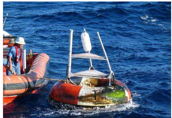
Figure 11. TAO Buoy Showing Damage from Removal of Components
