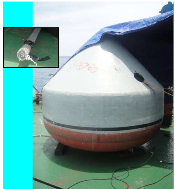
Figure 13. Cut Mooring Line on "Conehead" Anti-vandal Trial Mooring: Indian Ocean
