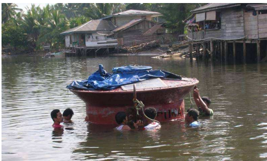
Figure 20. Indonesian Tsunami Buoy Recovery
