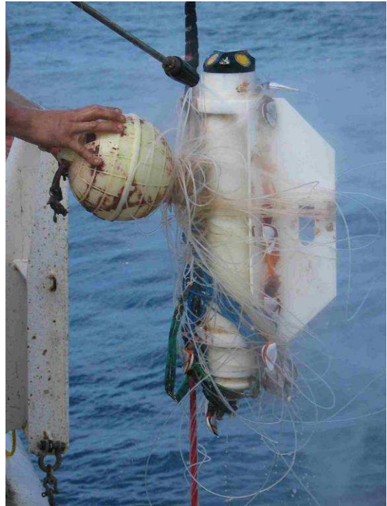
Figure 5. Fishing Line Entanglement - Subsurface Current Sensor (TAO Buoy)
