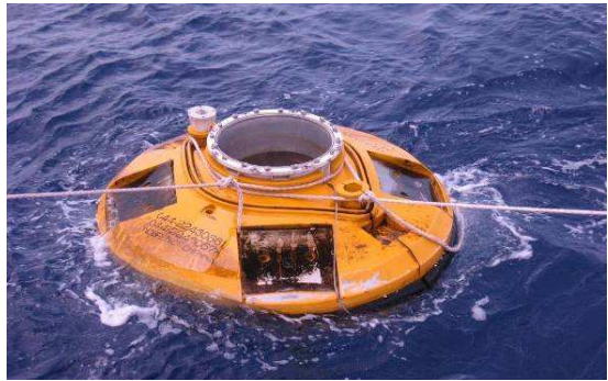
Figure 17. Indian Tsunami Buoy – Stolen Superstructure and Electronics Payload
