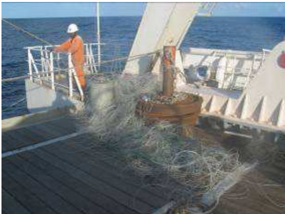
Figure 6. Fishing Line Entanglement of Mooring (Indian Ocean)
