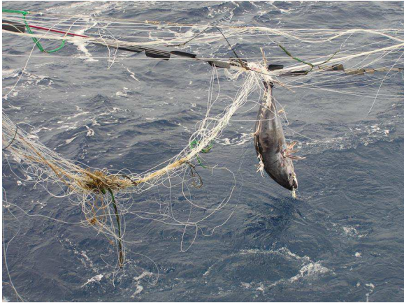
Figure 8. Tuna Fishing Gear Entangled on ATLAS Mooring (Indian Ocean)
