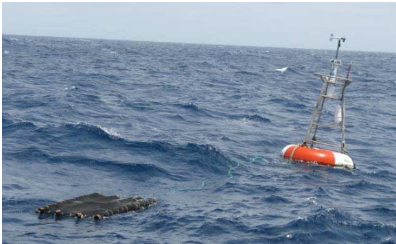
Figure 4. Fish Aggregation Device Attached to a TAO Buoy
