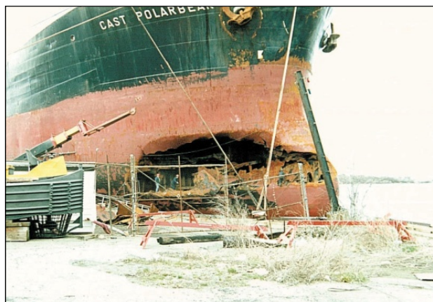
Damage from sea ice and icebergs is also an ongoing threat to shipping in high latitudes
