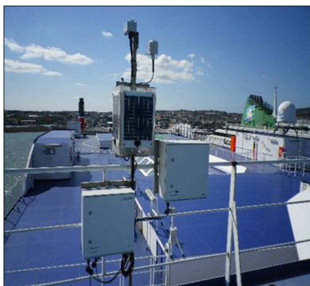
Observations from Automatic Weather Stations (AWS) allow for more frequent data transmissions. Supplementary manual observations by the crew are possible.
