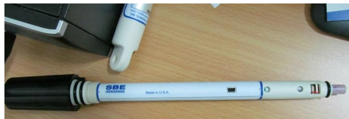
SBE-56 data logger with outer case removed prior to setup
