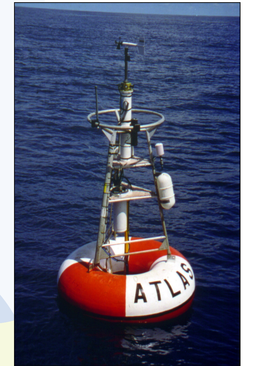
An ATLAS buoy, as deployed. Data are telemetered in real-time via Service Argos, and placed on the Global Telecommunications System (GTS) for assimilation into weather and climate forecast models
