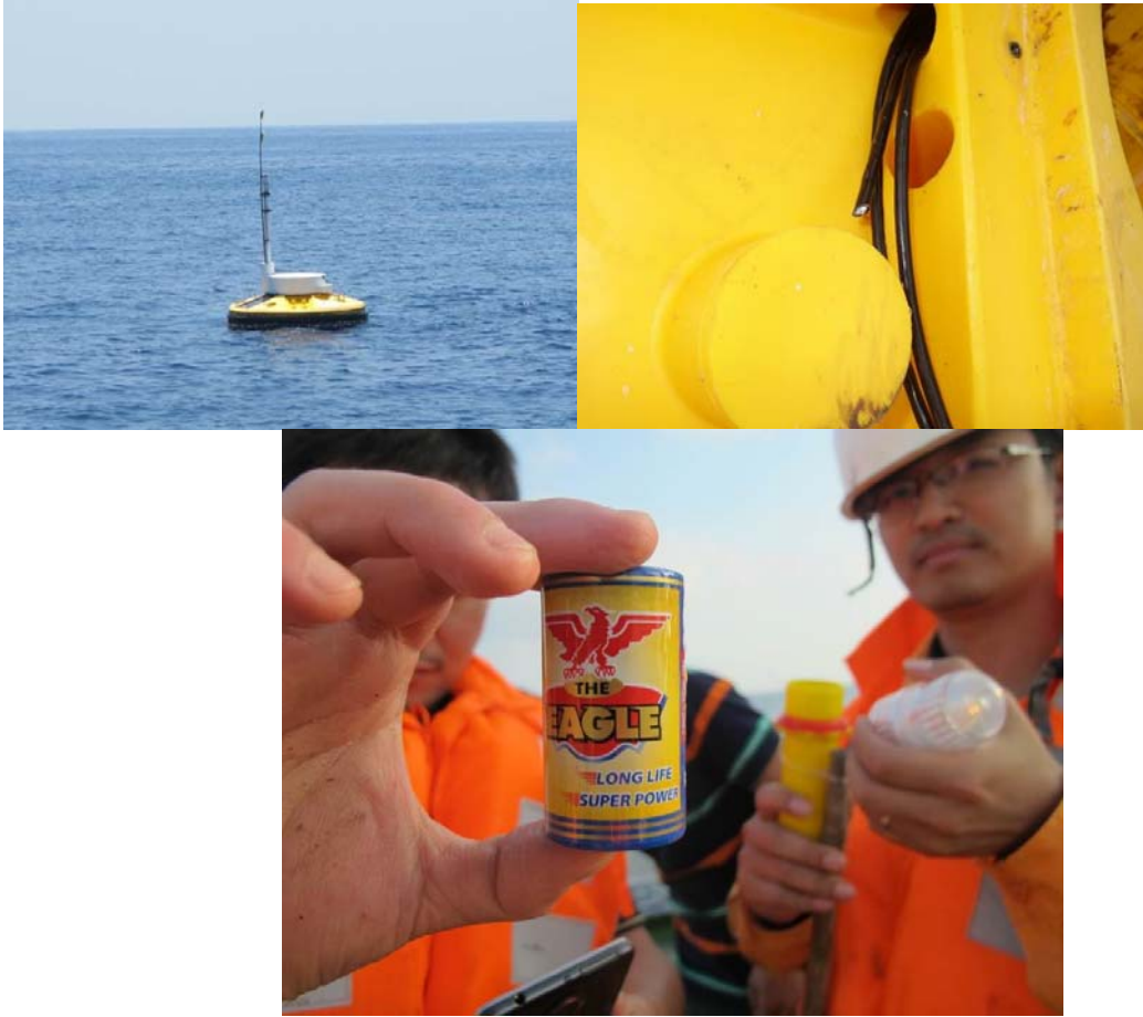
Figure 1 The damage of Tsunami buoys and the left battery
