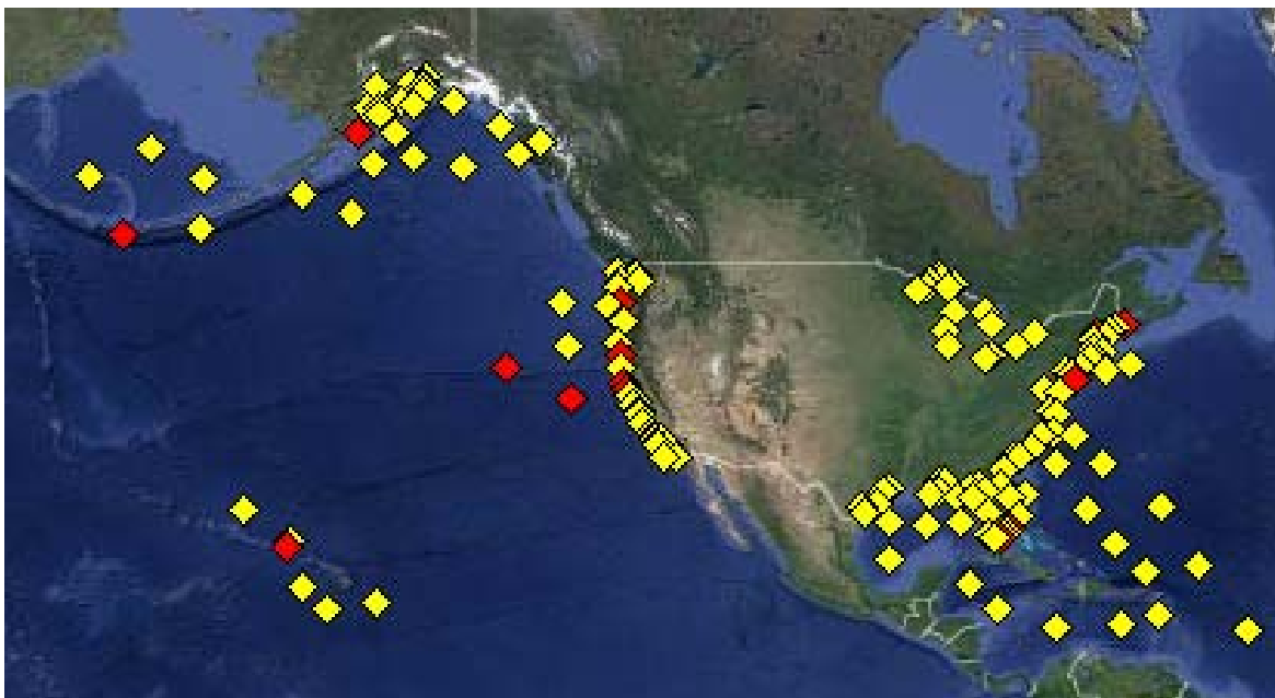
Fig. 3: NDBC Moored Buoys (MET/OCEAN), showing stations reporting in the last 8h (yellow) or not (red). Figure from http://www.ndbc.noaa.gov/obs.shtml . This image is for 20 August 2015.
