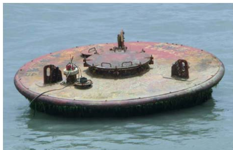
Figure3 Sensor lost and superstructure damage
