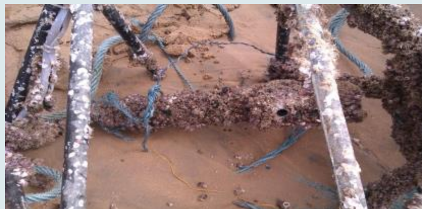
Fouled CT sensor
