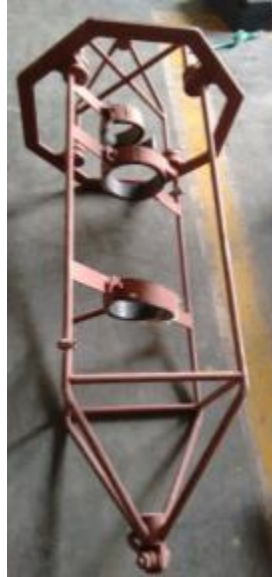
SS ADCP frame was painted with anti fouling paint
