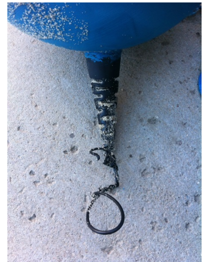
Broken 1/8" Spacelay Tether
