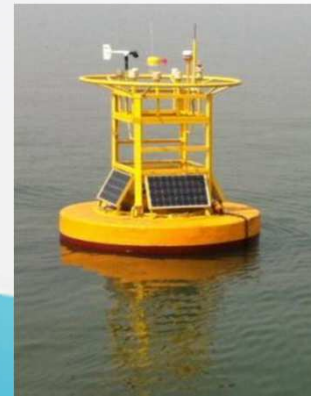
3m disc foam buoy
