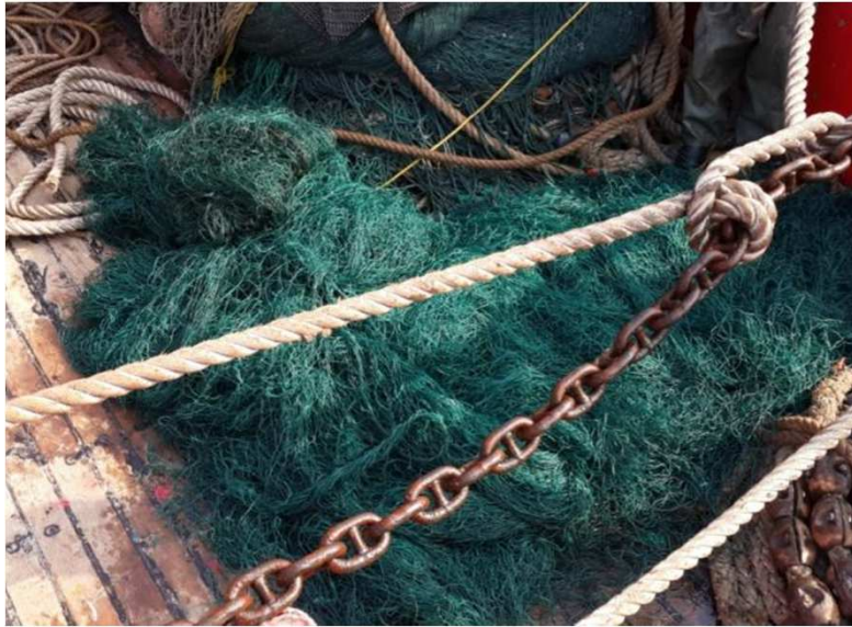
Fig. 6 Fishing line entanglement of mooring (2014.3.19-2014.3.22)
