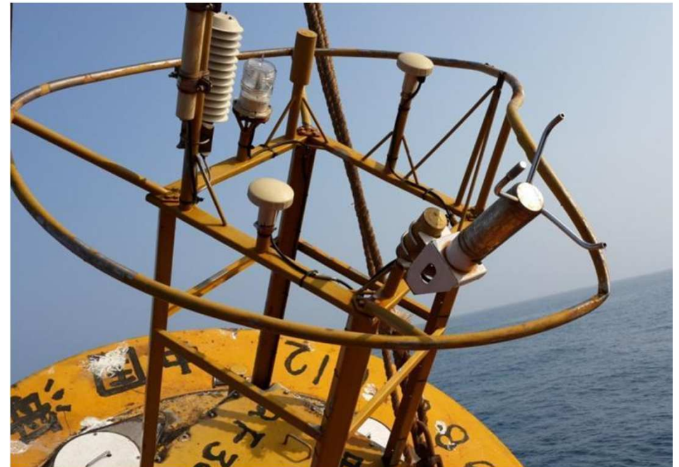
Fig.7 Sensor damage by collision (2014.3.19- 2014.3.22)
