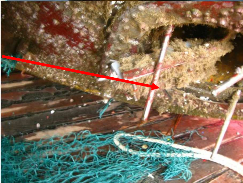
Fig. 5 Current meter probe lost (2014.2.18-2014.2.27)
