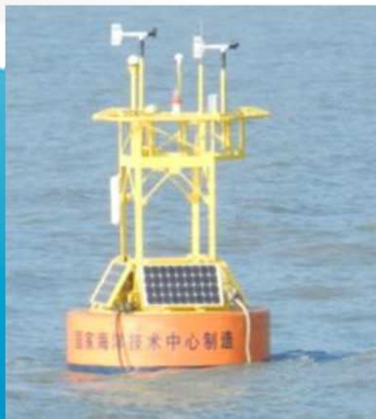
2.3m disc foam buoy
