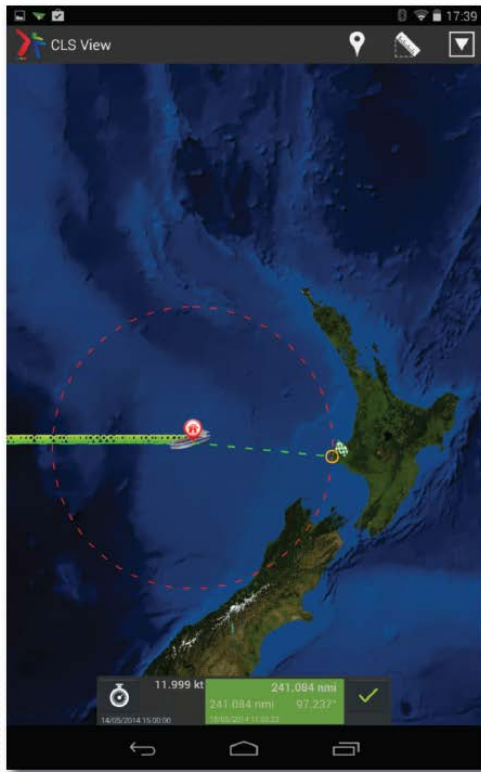
Distance measurements when in isoline mode take into account the curvature of the Earth's surface.
