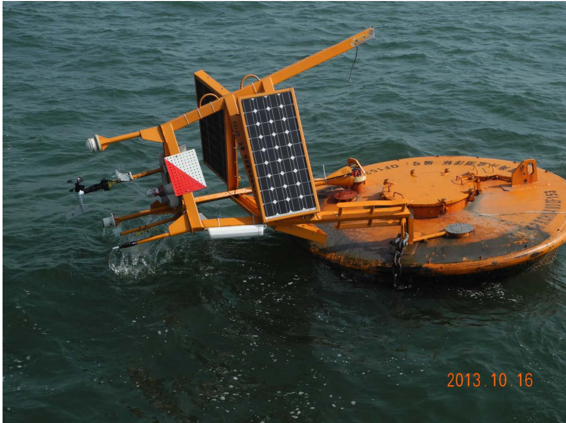
Fig.1 Ship collision damage to QF 153
