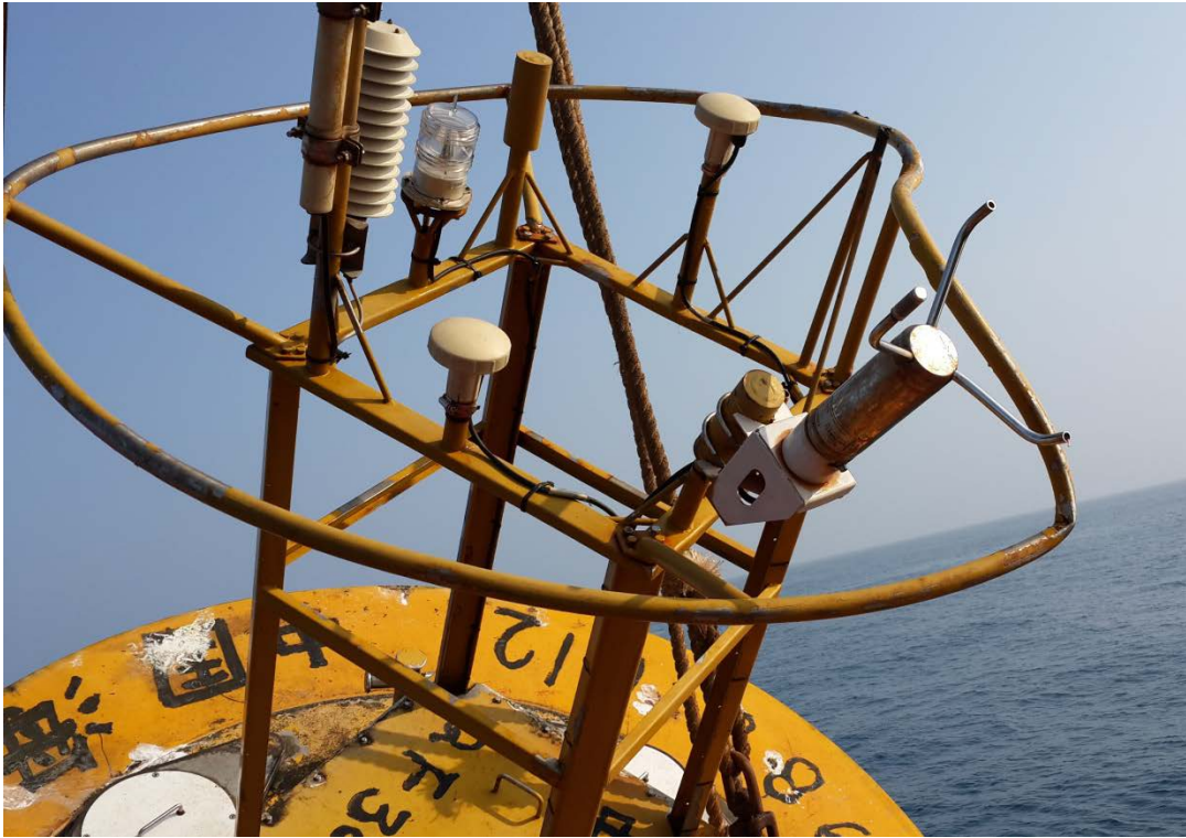
Fig.7 Sensor damage by collision (2014.3.19-2014.3.22)
