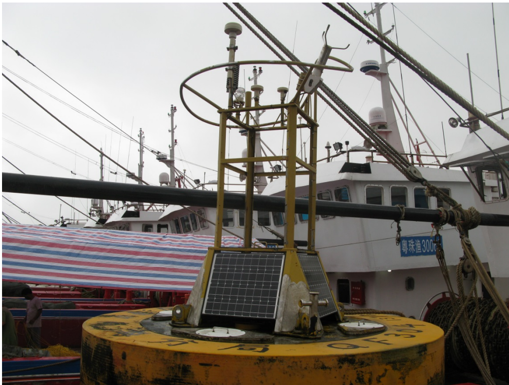
Fig. 8 Damaged buoy QF 304 by ship collision (2014.4.1-2014.4.5)
