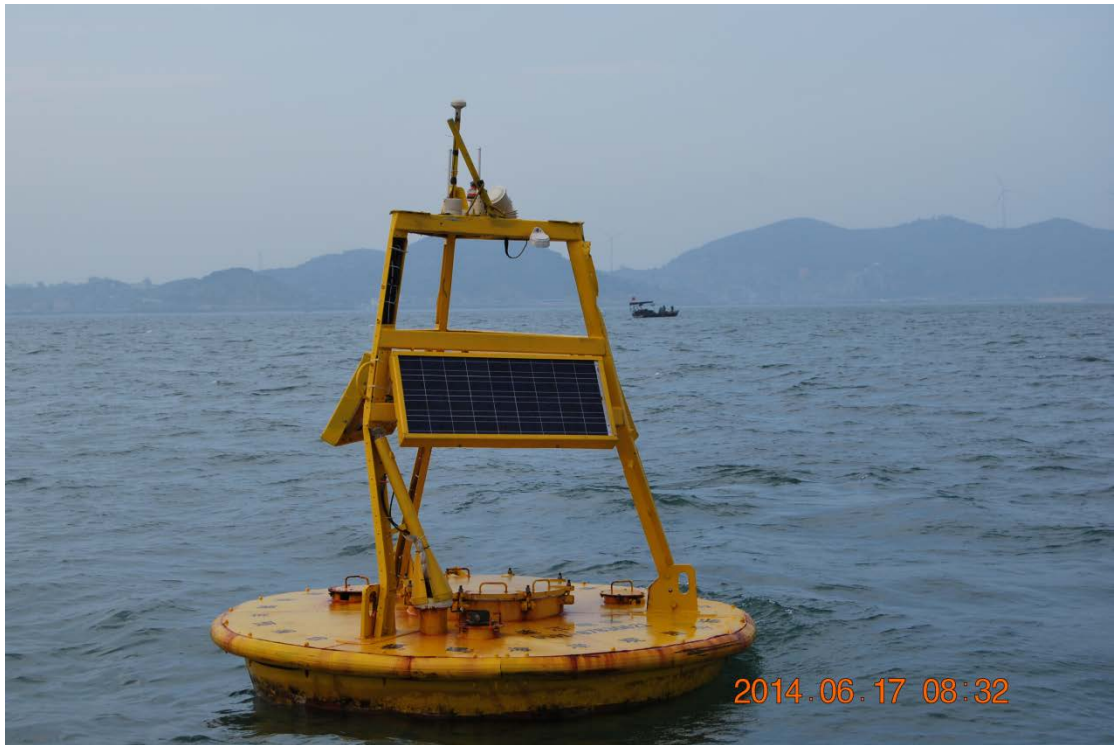
Fig. 3 Sensor lost and superstructure damage (2014.06)
