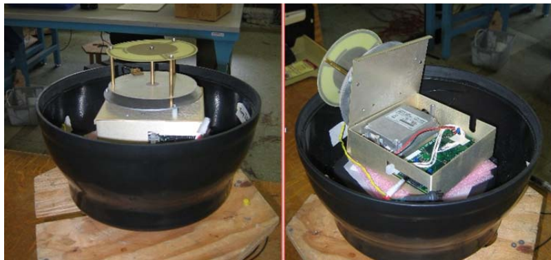
Figure 46 : Argos-3 Kenwood PMT integrated in a SVP drifter
