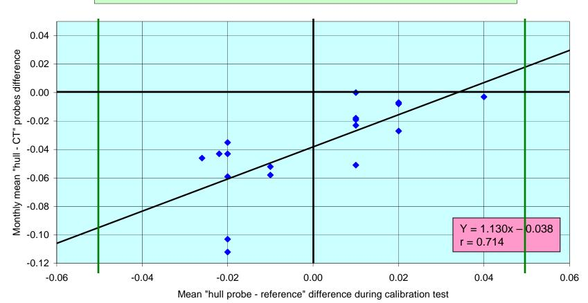
± 0.05K tolerance interval (calibration)
