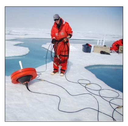
Preparing the thermistor string for playing through a hole augered into the ice.
