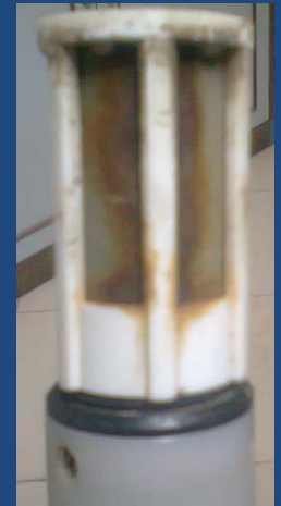
After retrieval Corrosion in the filter
