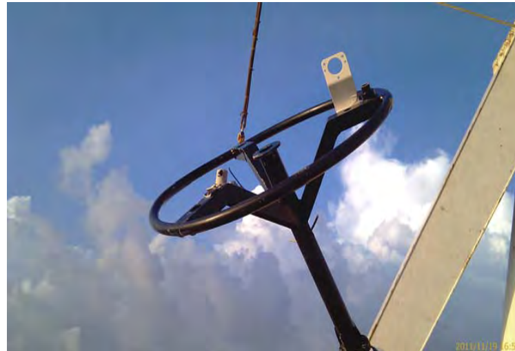
Vandalism BD13: Rainsensor missing. Bracket displaced, cable cut
