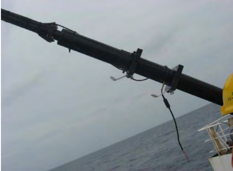
EPPLY Sensor is missing
