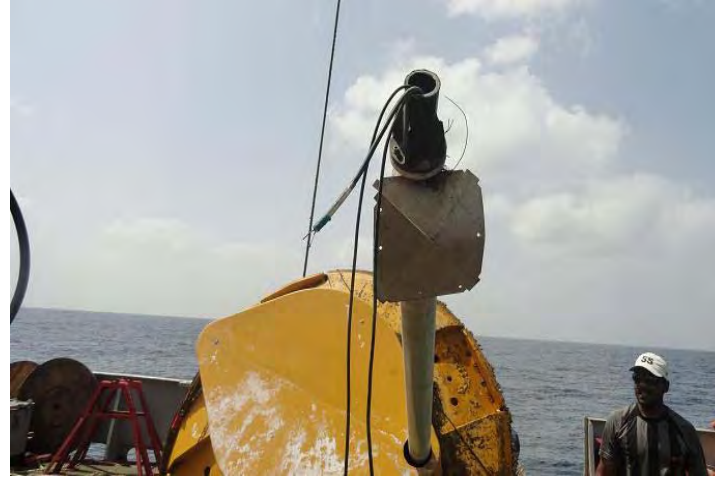
SW02 Buoy sensors and Antenna Vandalized
