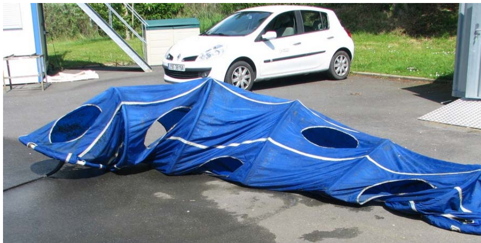
Figure 10. The view of SVP-BTC drifter’s drogue after it was cleared from one-year biology fouling.
