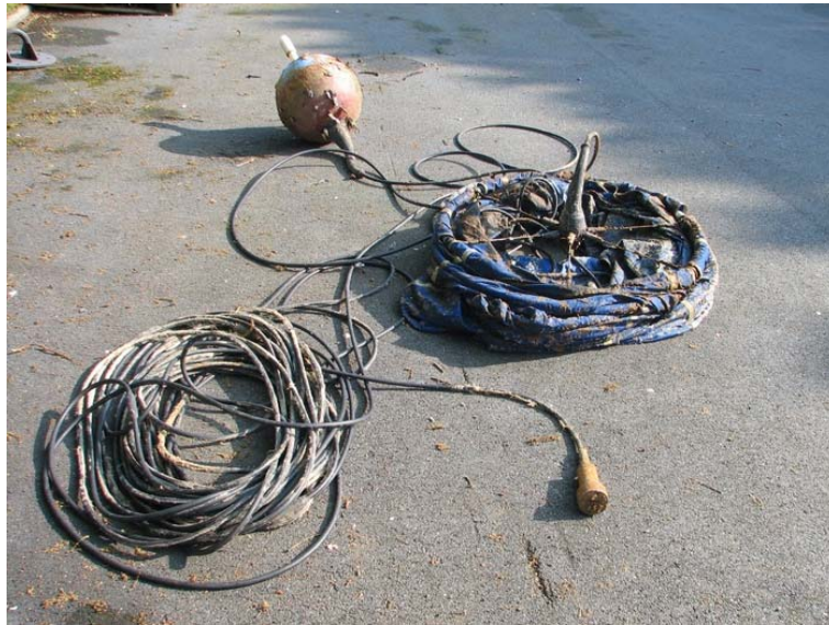
Figure 9. Main view of the SVP-BTC temperature-profiling drifter, which was recovered after one year operation in the Bay of Biscay.
