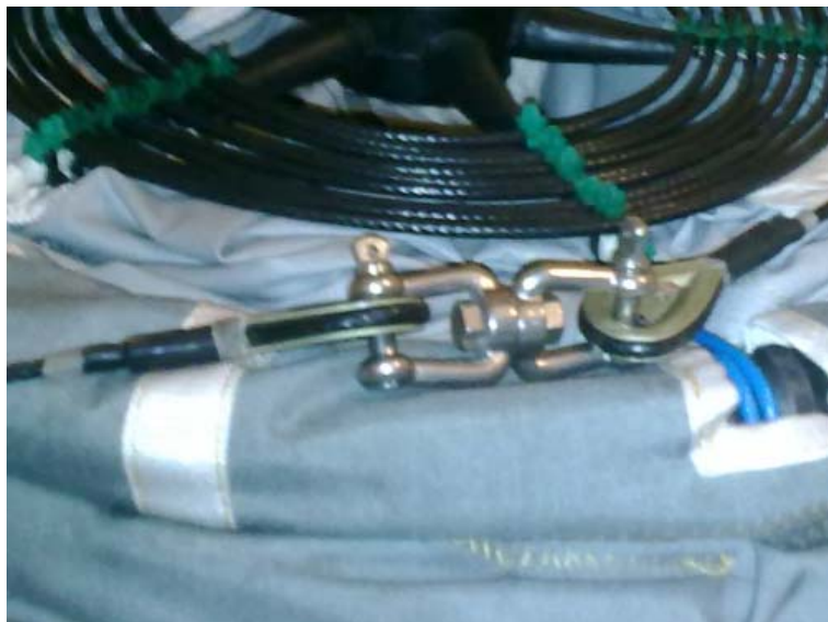
Figure 13. Swivel, inserted in tether below float to decrease influence of float’s bidirectional rotation on tether.
