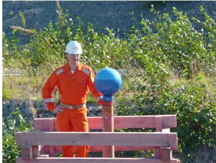
Figure 32. WLG-100 Water Level Gauge, fixed at the top of pipe liner of drilled hole.
