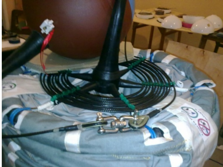
Figure 12. Spiral packaging of tether line in the clips, fixed to radials of “wire connection” to decrease probability of loops creation on tether during submergence of drogue after drop of buoy to water.
