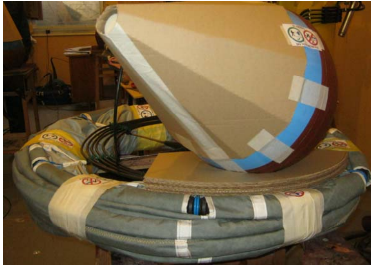
Figure 15. Main view of standard SVP-B drifter with 41-cm float and 92-cm drogue, prepared to be ready for self-deployment after drop to water.
