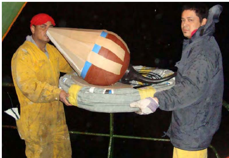
Figure 16. Deployment of the standard SVP-B drifter by means of drop to water from deploying ship.
