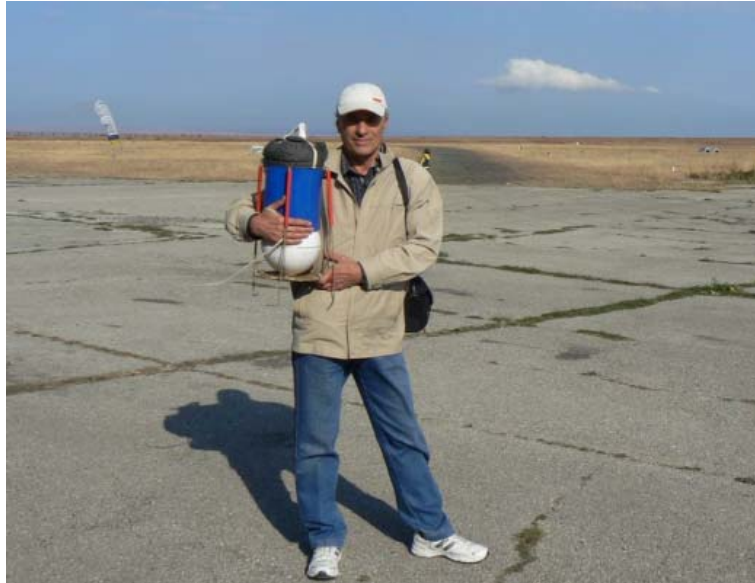
Figure 24. View of micro ice marker, equipped with parachute system to be deployed on ice or snow.
