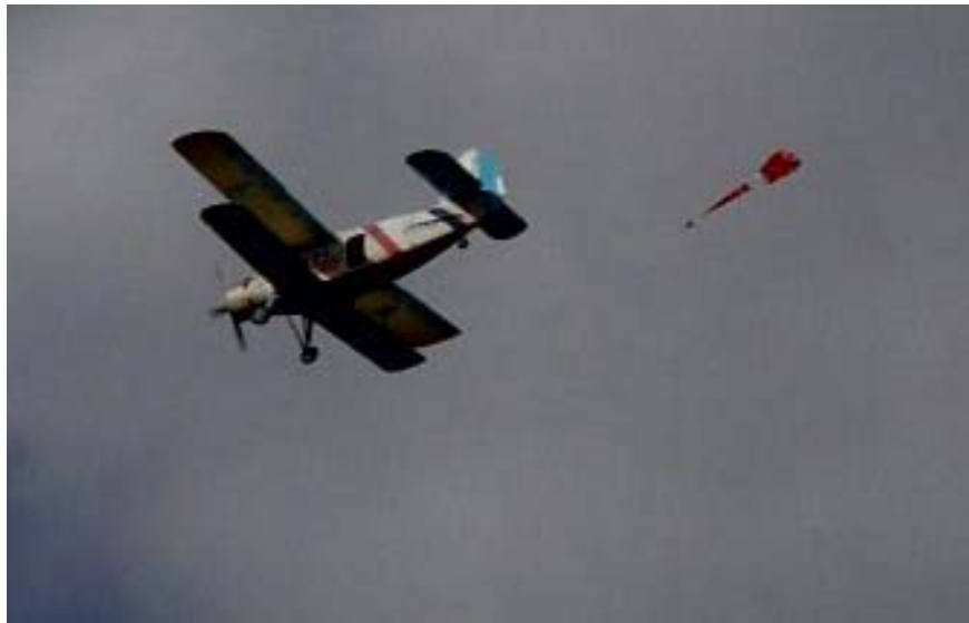
Figure 26. Opening of parachute after drop from aircraft.
