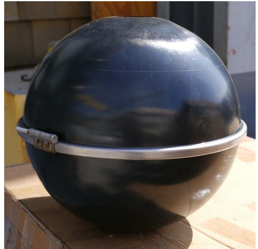
Figure: Injection molded re-sealable hull with sealing ring
