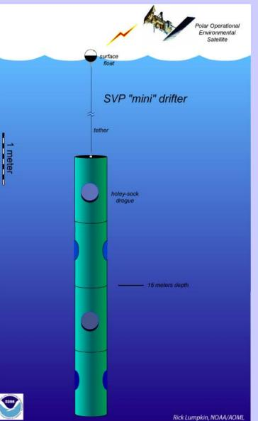
**Drogue (sea anchor):** provides 40:1 drag area ratio. Both original design and mini drifter are 40:1.
