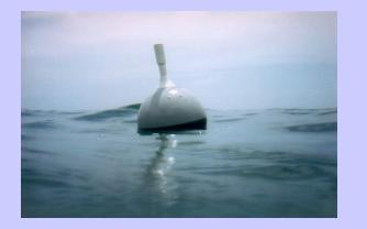
NOAA's Global Drifter Program: hourly measurements of nearsurface (15m) currents.
