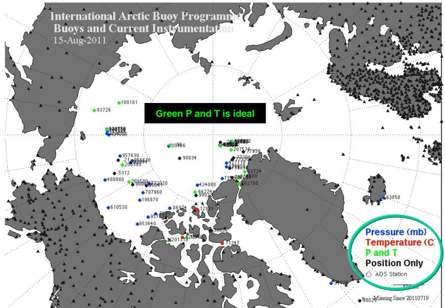
Several oceanographic buoys in array. Most also have basic air temperature and air pressure sensors and that data is getting on the GTS
