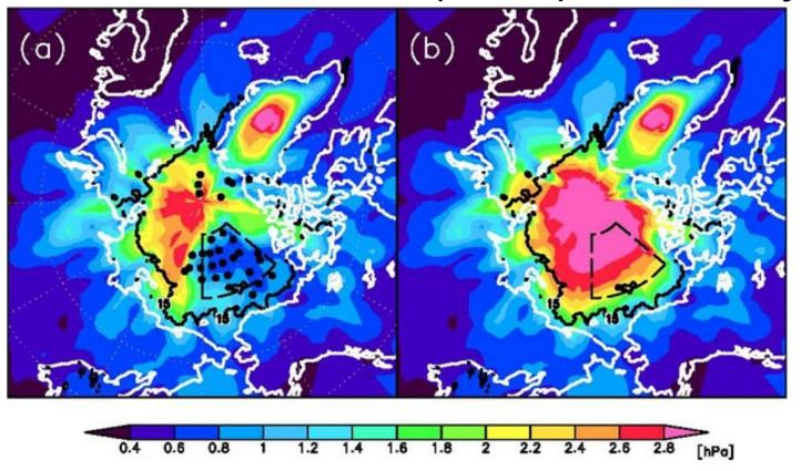
The spread between SLP Reanalyses is low in areas where there are buoy observations (left). The spread increases to cover the whole Arctic when the buoys are removed from the reanalyses (right). The buoy obs. also help constrain of estimates of wind and heat.
