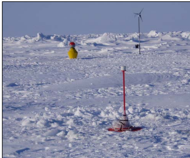
Polar Ocean Profiling System (foreground) & Ocean Flux buoy (yellow) Monitors Air and Ocean (typically deployed with IMB buoys)
