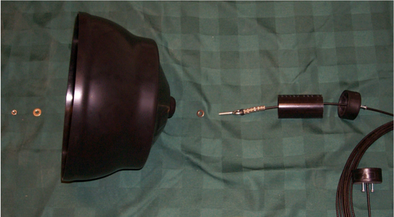
Figure 7. Connecting surface float to tether (top). Cap (bottom left), and eye-bolt (bottom right).
