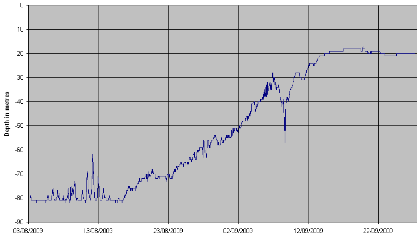
Marlin SVP-BTC drifter WMO 61690 Depth of the end of the thermistor string
