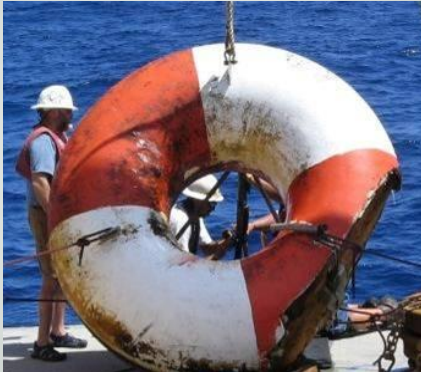
TAO buoy hull damage due to vessel collision
