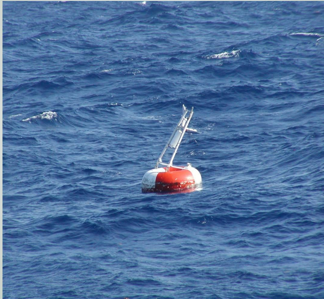
TAO buoy superstructure damage due to vessel collision
