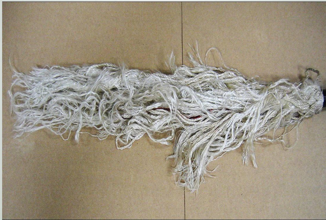
Tsunameter buoy vandalism: mooring line cut
