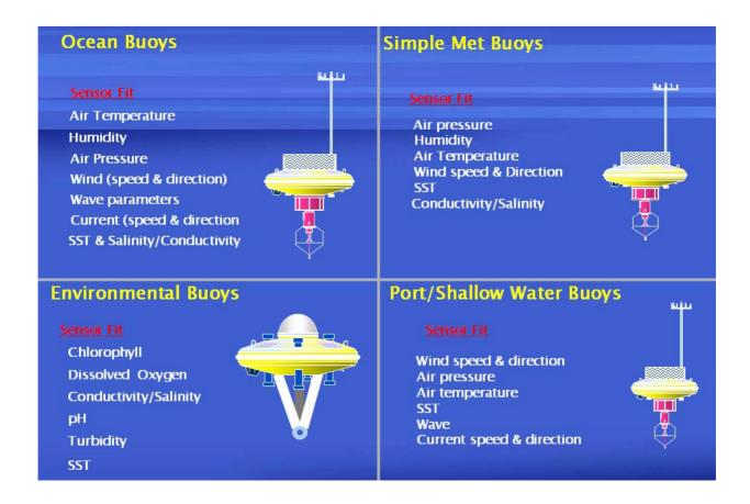
**Port Buoys:** This buoy is meant for shallow water locations closer to the predominant ports along the coast of India. These buoys are fitted with sensors such as Wind (speed & direction), Air Pressure, Air Temperature, Sea Surface Temperature, Wave and Current (speed & direction).
