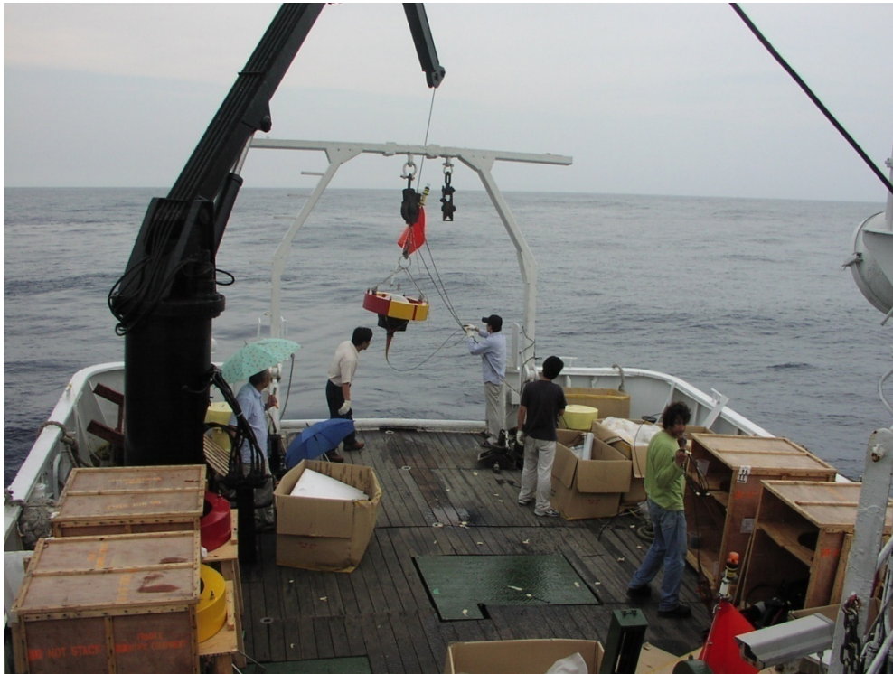
Deployment of a drifting thermistor chain from a small ship R/V “Ocean Researcher 2” in the South China Sea
