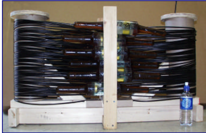
Figure 2 SmartSensor thermistor string. WOTAN pressure case is not shown.
