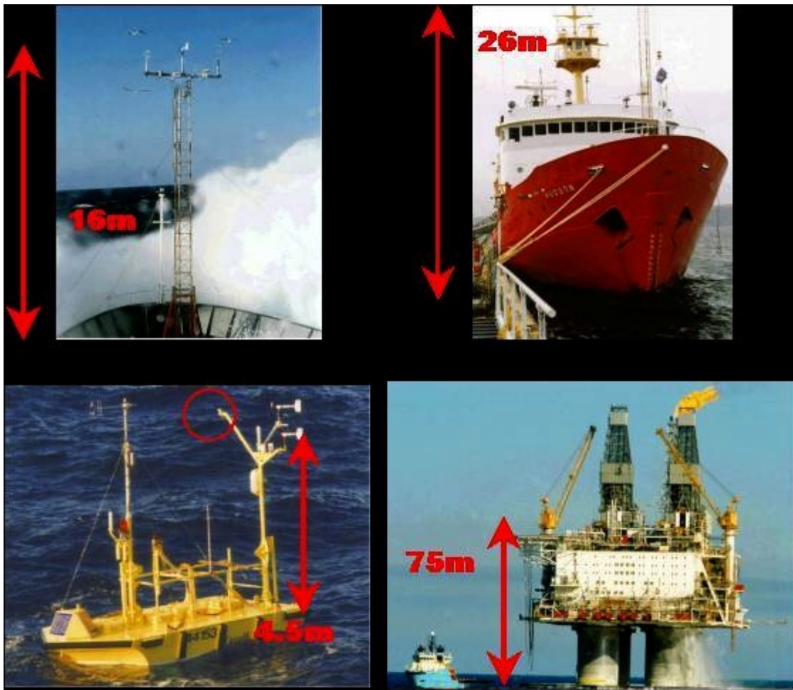
Figure 3. Comparison of the floating platforms geometry and instrument location: Hudson bowmast (top left), CCGS Hudson (top right), NOMAD buoy (bottom left) and Hibernia platform (bottom right).
