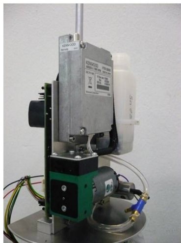
PMT integrated into a NEMO float
