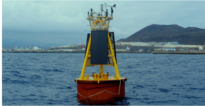
Moored buoy equipped with a PMT modem in the Canary Islands
