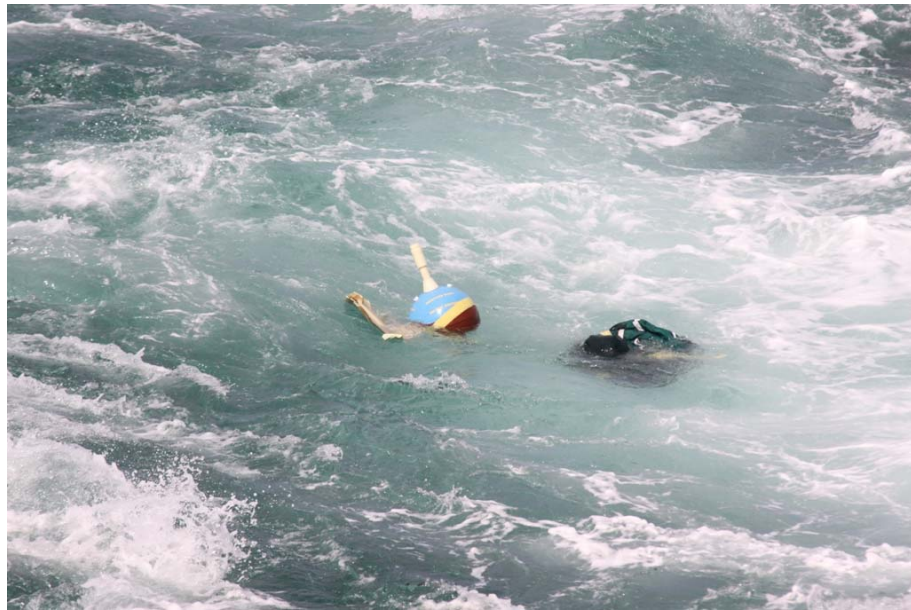
Figure 38 : Marlin-Yug Argos-3 SVP-B deployed in Tasman Sea (courtesy J. Fletcher)
