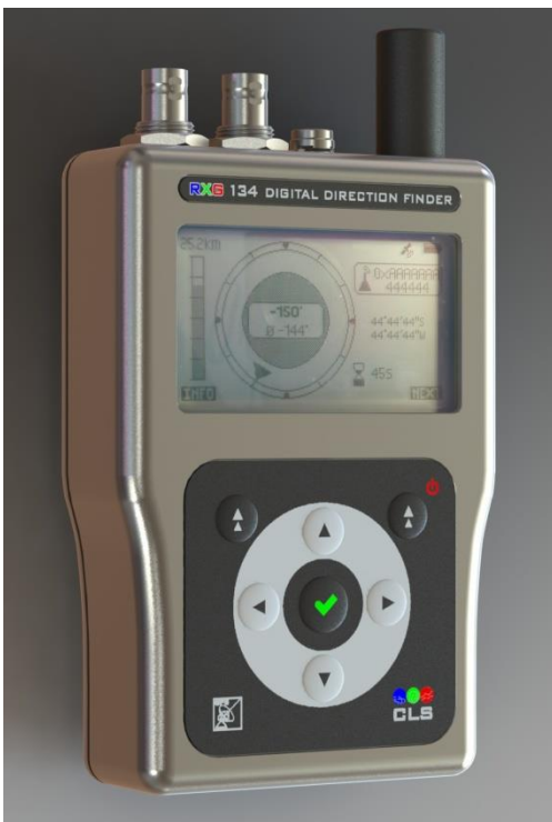
Figure 45 : New Argos goniometer
