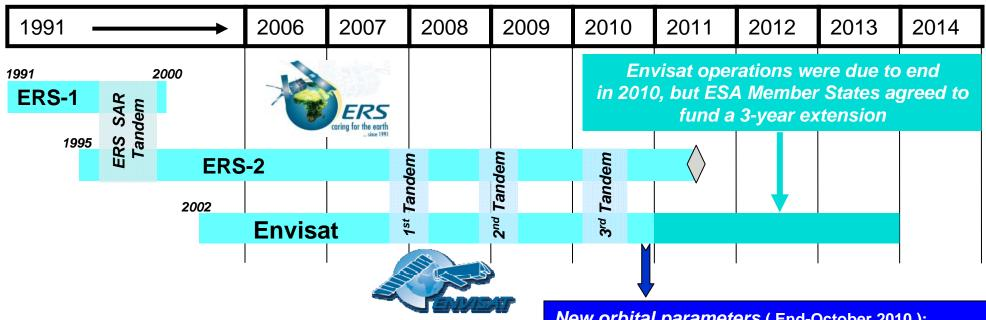
Efficient consumption of on-board hydrazine allowed operating nominally Envisat until 2010 (nominal 5-years lifetime ended in Feb. 2007), but most of hydrazine is now consumed.
