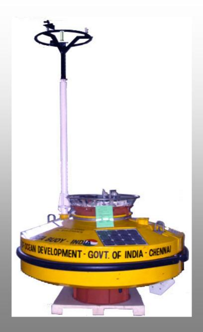
These buoys were not designed to measure/follow waves, they may roll (round hull), have resonances, or not respond well to waves...
