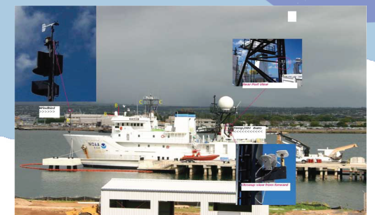
Figure 7: Side photo of NOAA vessel Ha'lalakai with sensor locations noted. A, B, and C marks are possible locations for air temperature, humidity, and pressure sensors recommended by SAMOS DAC.
