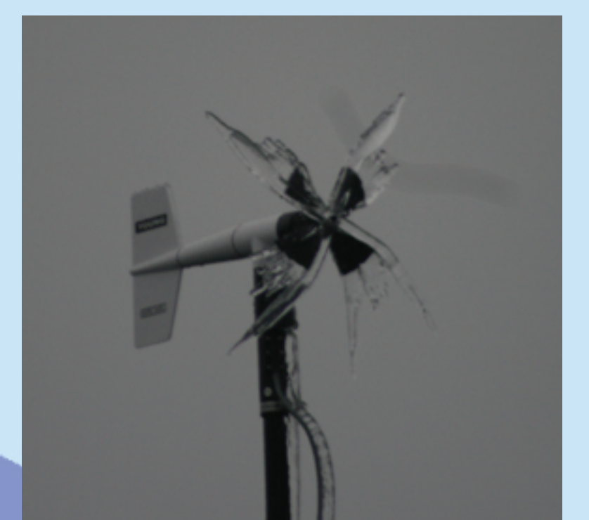
Figure 5: Frozen anemometer on the Oscar Dyson . Photo provided by onboard technician.
