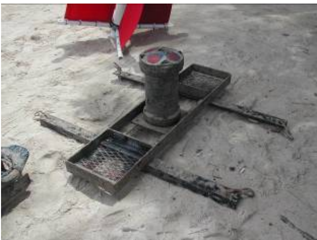
Frame-mounted Acoustic Doppler Current Profiler for Southeast Oahu Data Collection
