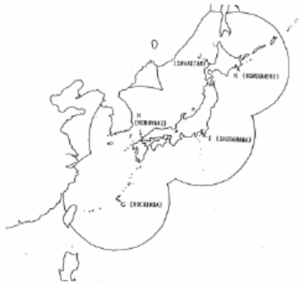
Fig.2 Area of responsibility for the NAVTEX of Japan and locations of the NAVTEX operation centers
