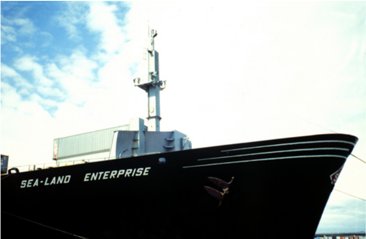
Figure 5 - Bow view of the SeaLand Enterprise. Bow mast with sensors is 70 feet above the deck.
