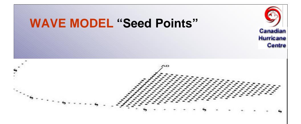
To reduce computational time, originating wave-points are pre-selected only for waves that "have a future," based on criteria for both wind speed and direction. The reduced, non-interacting wave point calculation set is determined by:
