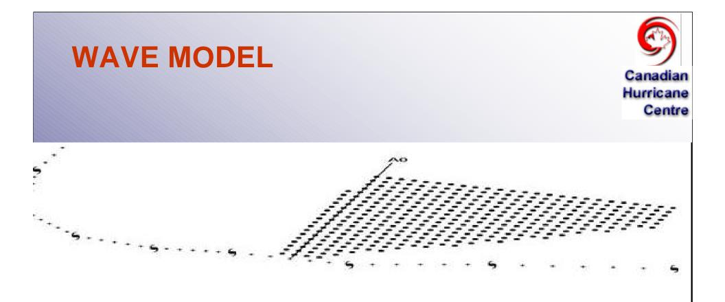
Waves from each initial calculation point are generated through successive time-steps until they are no longer supported by the local wind . . . they are then terminated.
