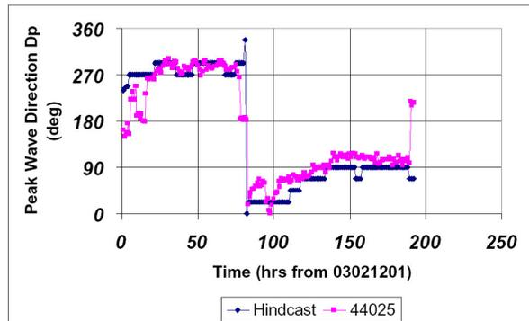
Figure 13. Wave direction comparison at offshore NDBC buoy 44025.
