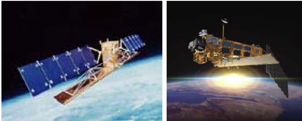
Figure 8: Radarsat-1 (left, launched in 1995) from CSA and ENVISAT (right, launched in 2002) from ESA are the two currently operational SAR missions.
