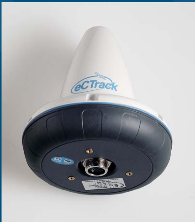
DCE/DTE (transceiver & messaging unit and GPS)
