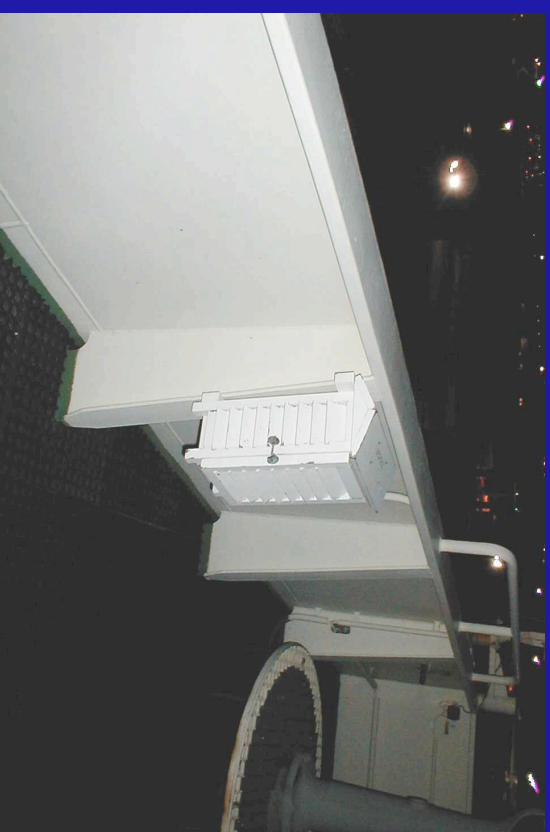
Poorly exposed screen
