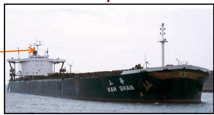
The ships are large 'block like' shapes which can distort the airflow above the ship.
