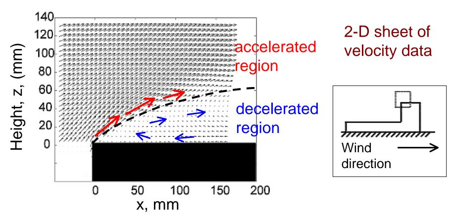
Anemometers placed close to the bridge top will experience severe deceleration and possibly flow reversal.
