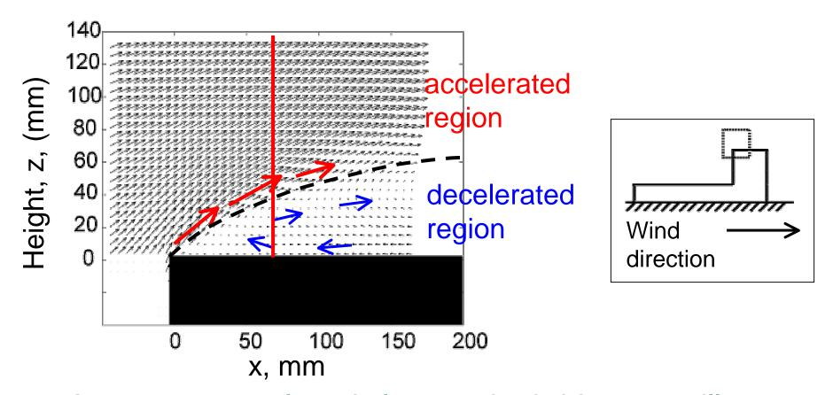
Anemometers placed close to the bridge top will experience severe deceleration and possibly flow reversal.
