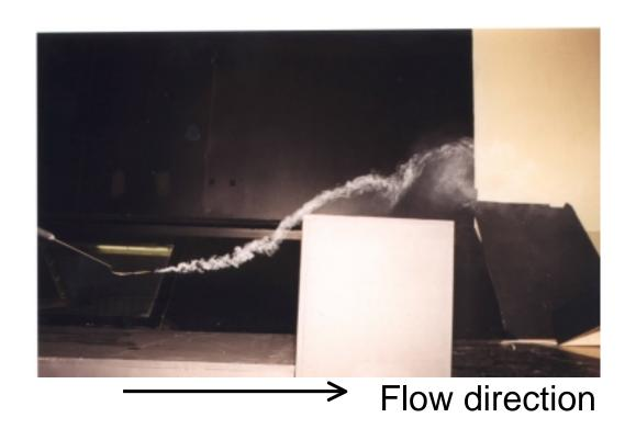
Basic flow visualisation of the airflow above the bridge of the tanker.
