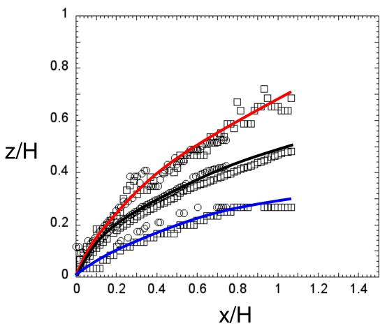
Using these simple relationships the sign of the bias can be determined for an anemometer position and bridge to deck height H
