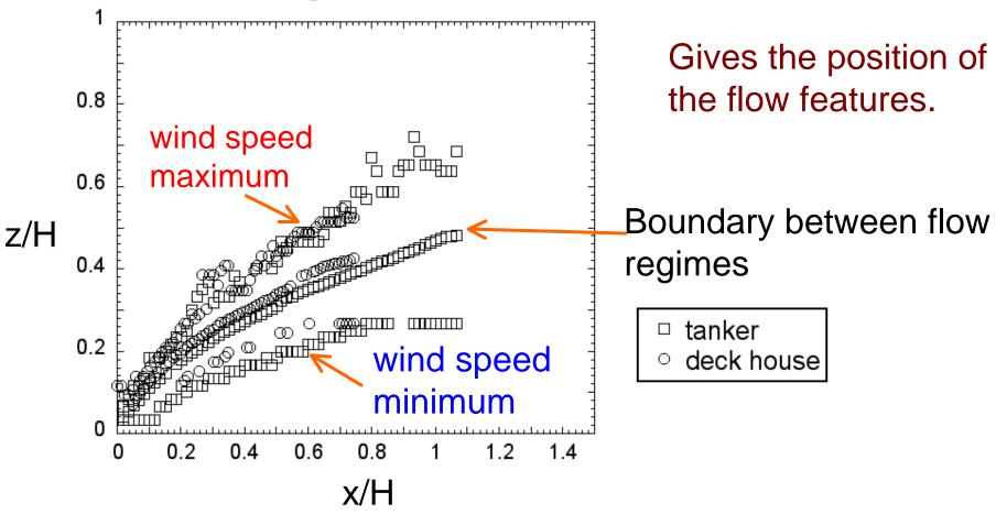
The important features of the flow field can be simply predicted from the bridge to deck height
