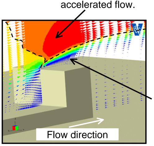
3D simulation of the airflow over the tanker.
