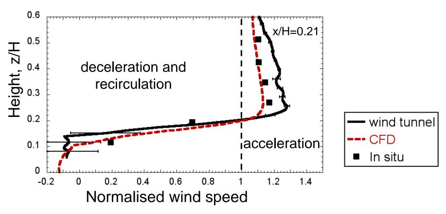
The wind speed can be biased high by 15 ±5%, or completely decelerated.
