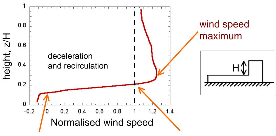
wind speed minimum (normalised wind speed=0)
