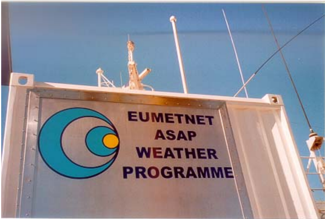
The E-ASAP launcher, here installed on the Mediterranean E-ASAP on the PELJASPER. The logo and text is in the upper 3 rd part of the stainless steel door with the launcher mounted on the inside.
