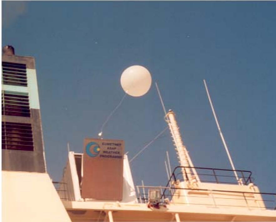
Figure 2. Radiosonde-launch from the E-ASAP container-launcher aboard the SEALAND ACHIEVER (WPKD). The container is situated at 30 m above sea level at normal draught. Note that the sonde has just left the launcher. The antennas are mounted on the roof of the launcher, but are here hidden behind the launcher door.
