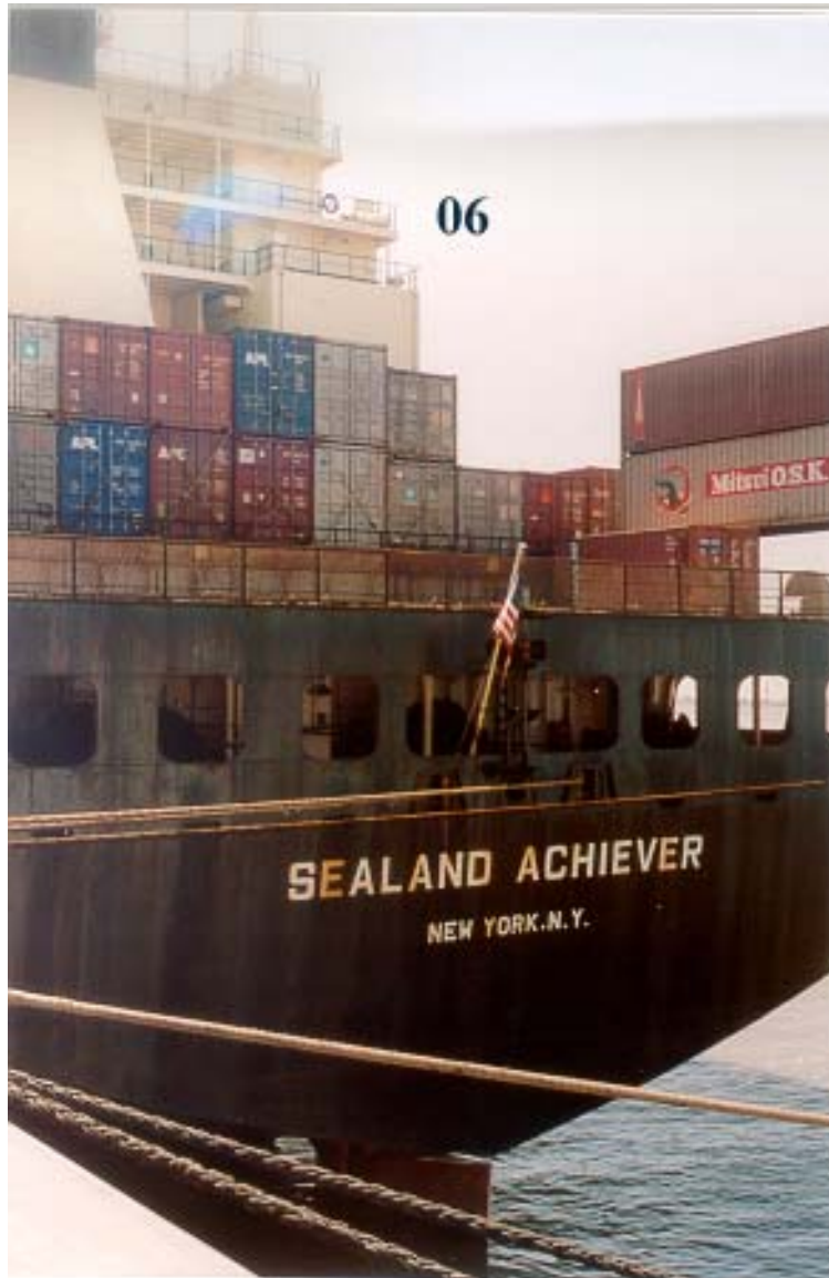
Figure 1. The SEALAND ACHIEVER seen from the stern before the E-ASAP container-launcher was put on the ship. It is placed on level 06 about 2 m to the starboard side from the funnel. The height above MSL of level 06 is 30 m at normal draught.
