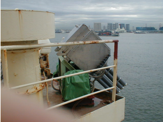
Photo 1. Automated XBT/XCTD launcher
