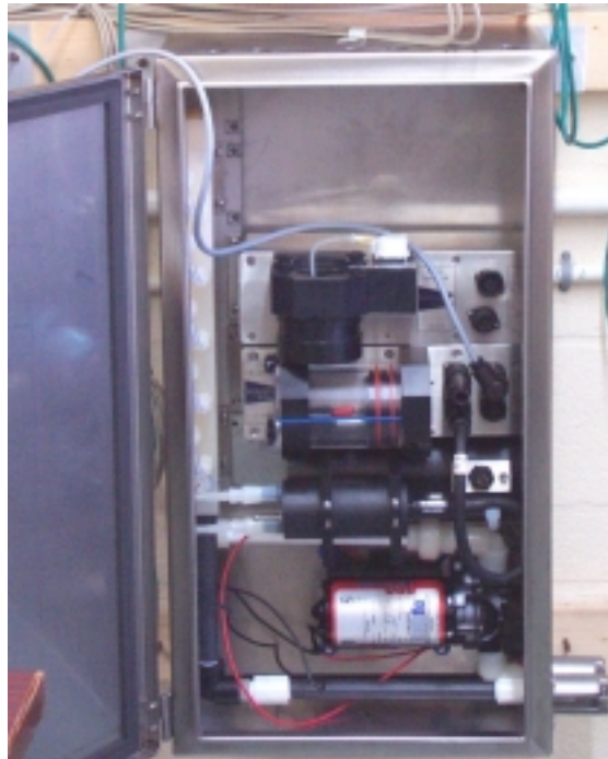
Figure 3. Instrument module with pump, manifold and 3 sensor submodules: Turbidity/CDOM, CTD (temperature, conductivity, dissolved oxygen, pH, Eh), and a prototype trace metals analyzer.
