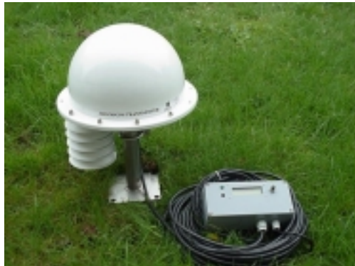
Figure 2: Minos : self-contained Argos telemetry station with atmospheric pressure, air temperature sensors, GPS, and data display unit for crew members.
