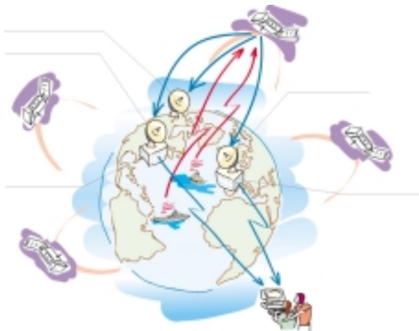
Figure 1: Argos is flown onboard the NOAA polar orbiting satellites (5 satellites as of today), and will also fly on NASDA and EUMETSAT polar orbiting satellites.
